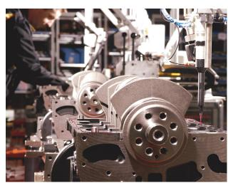
The highly automated Dove Valley factory uses a robotic machine to apply a precise bead of sealant to the bottom of the block before the bedplate is installed.
