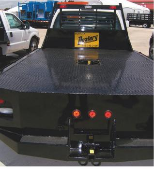
A stout, steel flatbed can carry cargo or, with its gooseneck hitch uncovered, pull a trailer weighing up to 16,700 pounds.
