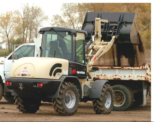
("speeder") system allows a top end of 22 mph, versus 12.4 mph for the standard system. The speeder option is advantageous, says Georg Seyrlehner, global product marketing manager, if the unit is frequently driven between work sites or is used on large developments to deliver materials or to make relatively long load-and-carry runs.
