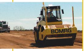
The Minnesota Department of Transportation has been investigating intelligent-compaction soil machines for the past two years and continues to do so. The Bomag (pictured), fitted with the company's Vario-Control system, was set up to run with a GPS-based documentation system on the Minnesota site.
