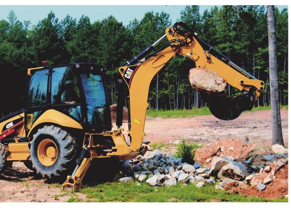
Caterpillar redesigned most of its frame structures, including switching to an exterior-sliding extendable dipper stick that made way for secure mounting of bucket thumbs at the factory.
