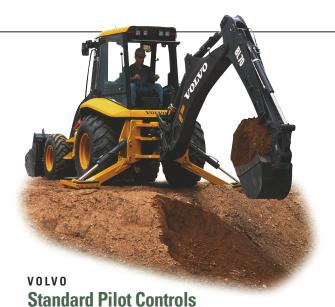
In January, Volvo made pilot hydraulic controls standard equipment on the BL70, with mechanical controls available as an option. A new loader-control joystick features a proportional switch for auxiliary hydraulic control. The standard loader features a center-mounted bucket cylinder, but this year brings a new toolcarrier option for the loader featuring parallel lift and a hydraulic quick coupler for changing attachments.
