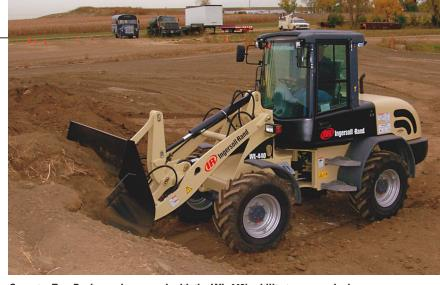
Operator Tom Rush was impressed with the WL-440's ability to aggressively engage a reasonably tough stockpile without wheel spin. Axles feature a limited-slip differential, which automatically transfers power to the wheel with better grip. The machine also has a brake/inching pedal that allows the operator to control ground speed irrespective of engine speed.
