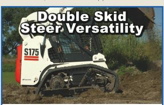
Get the versatility of two machines in one when you add the Loegering Versatile Track System™ (VTS™) to your current skid steer. The VTS suspended rubber tracks gives you significantly more floatation, stability and traction.
