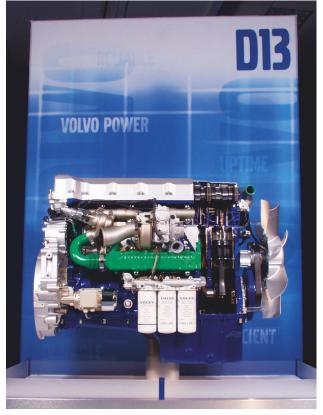
Volvo expects its upcoming D13 to be its highest-volume '07 diesel. It will be used in VN highway tractors and the only engine offered on the VHD vocational series. The D13's eight ratings range from 335 to 485 horsepower.
