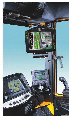
The cab of this Bomag BW213-4 BVC roller, which is fitted with the company's VarioControl system — an IC system for soil machines, incorporates the machine's basic control panel (center), the VarioControl operating panel (lower right) and the Bomag documentation system (upper right).
