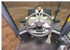
The expansive front window of the WL-440 provides a good view to the bucket and work area. Controls are straightforward once understood. A switch at the lower left of the panel locks out implement hydraulics — a safety feature. When activated, the lockout disables the joystick, including directional shifting capability, but a switch next to the lockout allows shifting the machine to permit travel.
