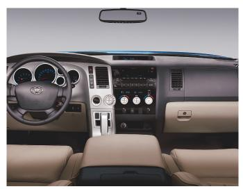
New Tundra's roomy interior will come in Base, SR5 and Limited (shown) trim packages. Large HVAC knobs are designed to be worked with a gloved hand.
