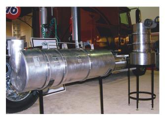
Horizontal and "compact" vertical diesel particulate filters will trap engine soot and ash, and double as mufflers. Both Volvo and Mack will use these exhaust aftertreatment devices.
