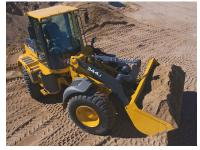
more stable maneuvering under load. The standard return-to-dig feature automatically returns the bucket to a preset level. Closed-center, load-sensing hydraulics eliminate power waste, and control-lever efforts are easier and more precise with excavator-style controls.
