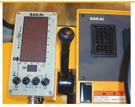
According to Sakai, the basic operating principle of its IC models is that of adjusting amplitude, and the stiffness values reported by these units will be based on a measure of the material's "dynamic modulus."
