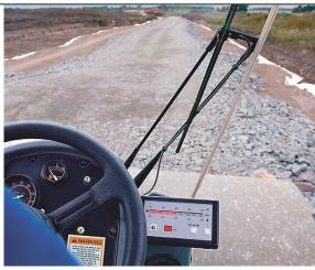
The Geodynamik CompactoBar provides a continuous value relative to material stiffness. The basic technology behind this instrument is at the heart of today's intelligent-compaction systems. In the early 1990s, Geodynamik developed an IC system that adjusted not only amplitude and frequency, but also machine speed. The idea lost momentum, says Carl Pettersson, the company's managing director, because of market indifference and the cost of electronics at the time.
