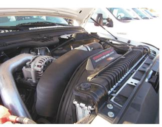
Under all the shrouds, pipes and accessories is the PowerStroke V-8 diesel, which makes as much as 325 horsepower and 570 lbs.-ft. So the truck really scooted and was clean-burning to boot.
