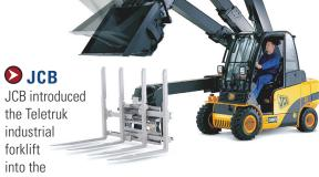
North American market. It is a two-wheel-drive hydrostatic machine that uses a telescopic boom not a vertical mast. It has a load capacity of 7,000 pounds. JCB says the telescopic-boom feature provides forward reach that enables the Teletruk to perform where a vertical-mast forklift cannot.
